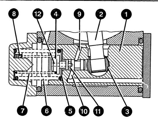
COMPONENTS OF TIMING DEVICE WITH NO FOLLOWER PISTON (Standard timing device)
